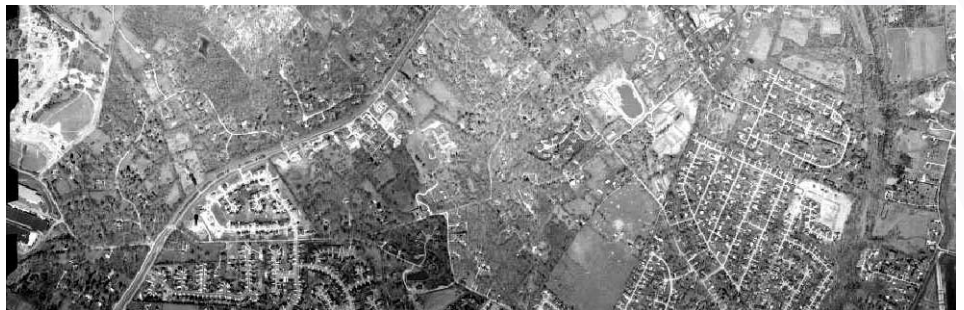
Although photos are flat, our world is not. LOJIC staff, with the help of local engineering firm Fuller, Mossbarger, Scott and May, has converted aerial photos used for LOJIC maps into three-dimensional images called orthos, which correct distorted photos by taking into account the earth's curvature and elevation. The resulting mosaic of images together creates a seamless picture of our community as photographed from the air. The process allows computer viewers to zoom in and out of specific locations, making LOJIC maps more meaningful and user friendly.
