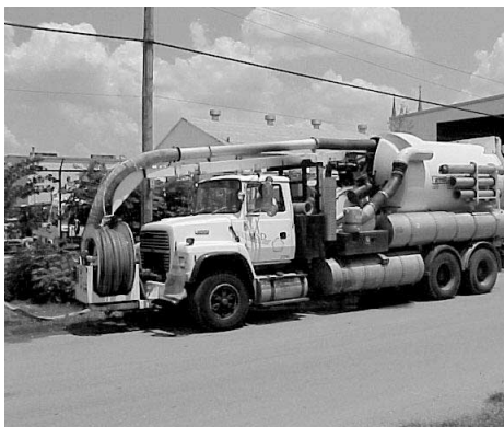
MSD uses a vactor truck like this one to clean catch basins, like the one near Ms. Edwards' Camp Taylor home.
