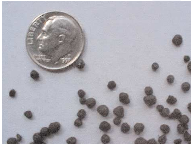
Dried biosolids are in small pellets ranging from one to four millimeters in size with 95 percent of the liquid removed.
