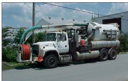
MSD's fleet includes non-driveable equipment (like generators and pumps), sedans, vans, vector trucks (shown above) and other vehicles.
