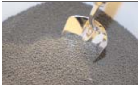
Dried biosolid pellets from the alternative solids process may be used as a fertilizer in the future.
