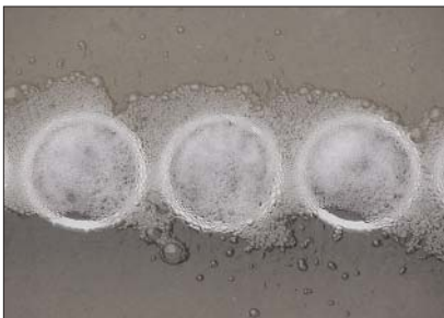
Fine bubble aeration provides improved biological treatment of wastewater and significantly reduces odor emissions.
