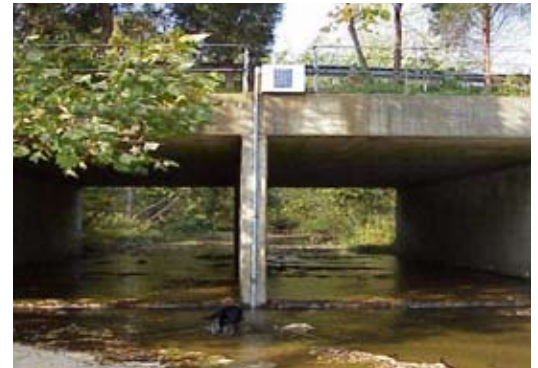
Data reported electronically from 24 stream monitoring locations in Louisville Metro allows MSD to quickly respond to changes in water quality.
